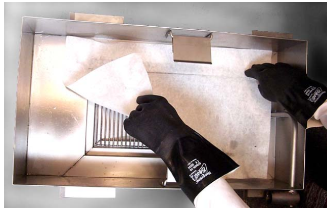
Placing filter screen (pan grid) in filter pan.
